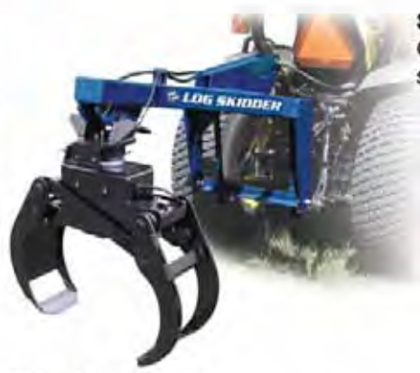
SB06 Log Skidder Three-point hitch grapple attachment for tractors in the 20-60HP range
